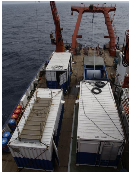
Fig. 3. View toward the stern on the working deck of the research vessel Meteor during deployment of the MeBo. In front are the workshop and control containers, behind them the drill pipe storage and winch, and behind those the launch and recovery system for the MeBo (Photo: V. Diekamp, MARUM).
