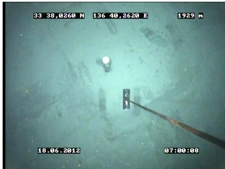
Fig. 8. Picture of a MeBo-CORK installed in June 2012 with MeBo off the coast of Japan. The picture was taken a few days after installation with a towed camera sled, the Ocean Floor Observation System (OFOS) of the research vessel SONNE . Note the imprint of the base frame and of the legs of the MeBo on the sea floor. The distance weight on a 2 m rope at the lower right of the picture belongs to the camera sled and assists the winch driver in assessing distance to sea floor (Photo: MARUM).
