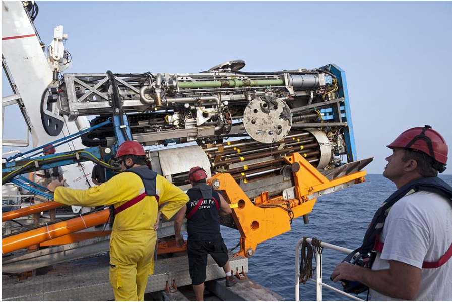
Fig. 2. The sea-floor drill rig MeBo during the deployment start from the research vessel R/V POURQUOI PAS? in November 2011 (Photo: T. Klein, MARUM).
