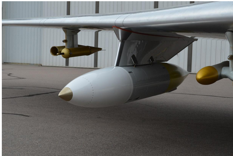
Figure 1. View of NCAR pod mounted below surface of right wing.
