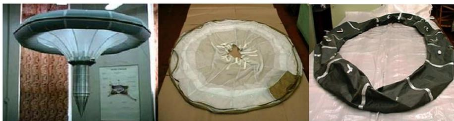
**Fig. 6.** Inflated Additional Inflation Breaking Unit ( T-IBU) shown on the left with the Surface Module (SM). In the center the cover of the T-IBU and on the right the gas tight bladder.
