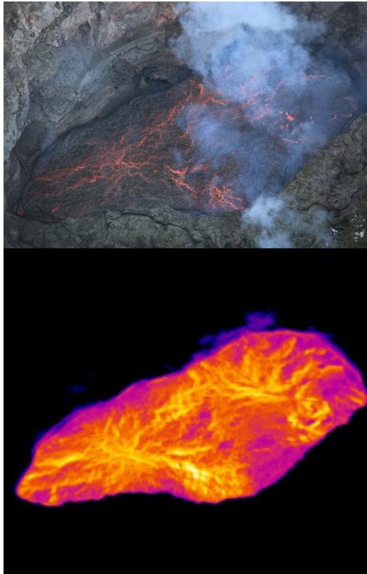
**Fig. 5.** Simultaneous images from a digital SLR camera and the IR camera. The cracks in the lake's crust are clearly visible in the IR image and can be used to estimate the surface motion of the lake. The ability of the IR camera to image through the volcanic plume is also clearly demonstrated.
