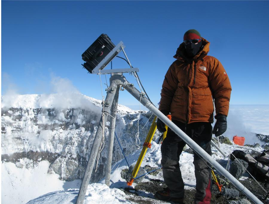
**Fig. 3.** The new thermal camera system installed at the crater rim of Erebus volcano.
