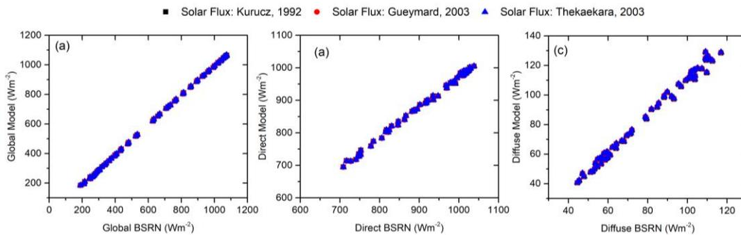
Figure 1. Scatterplot of the instantaneous ( $Wm^{-2}$ ) radiation measurements and simulations for (a) global, (b) direct and (c) diffuse radiation considering three extraterrestrial spectra.
